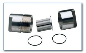
The 6300 Series Filter provides reliable filtration in a compact inline configuration. The filter element is made up of seven (7) porous cups, which substantially increases the area over traditional designs, and ncreases on-stream filter life. The filter surface area is 10 square inches.
